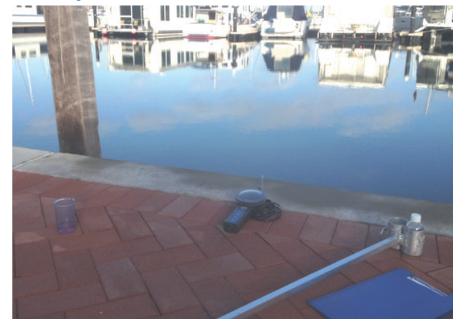
Figure 3.7 Mandurah Ocean Marina Site: handheld water quality metre, sampling bottle and clipboard
